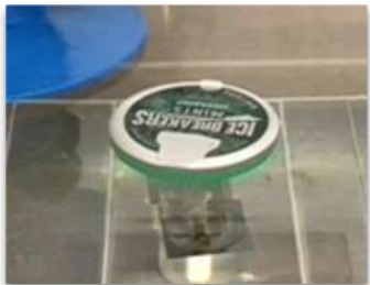
A reference target (plastic void candy box) of 7.5 cm diameter.
